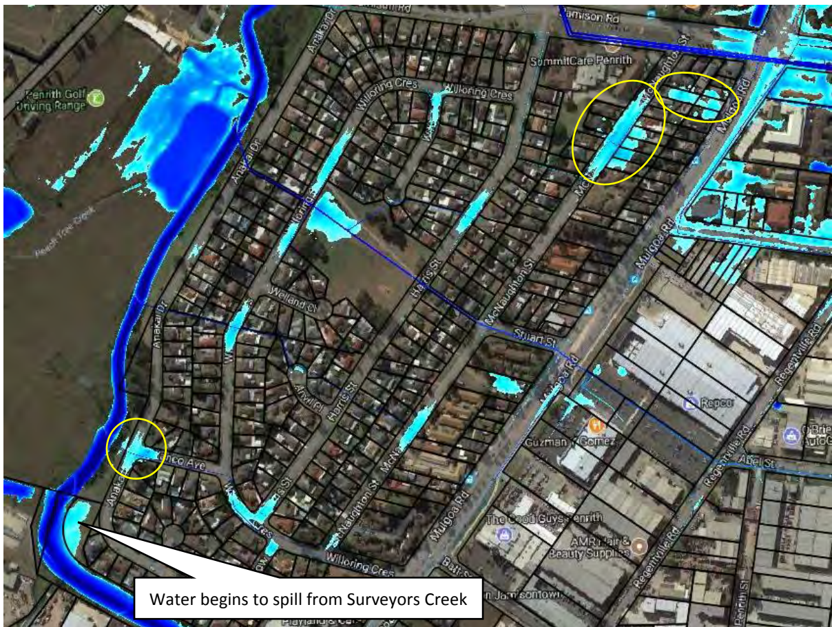
Plate 31 1% AEP Depths near Anakai Drive and McNahughton Street after 110mins of rainfall.
