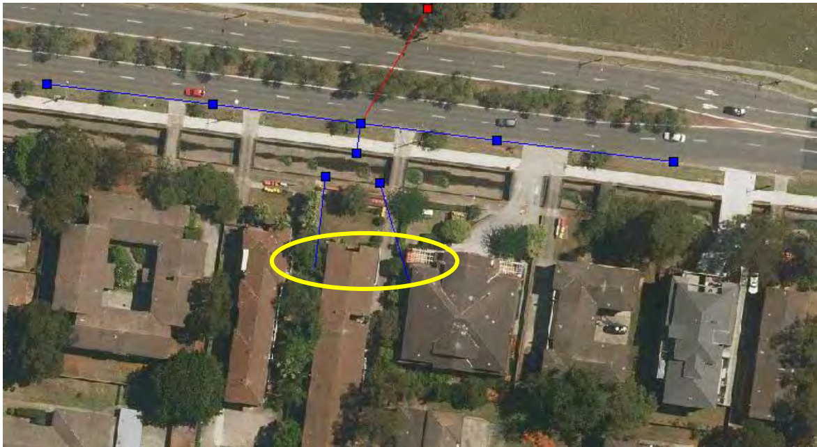
Plate 2 Example of stormwater pipes on private property with no upstream connections/pits
