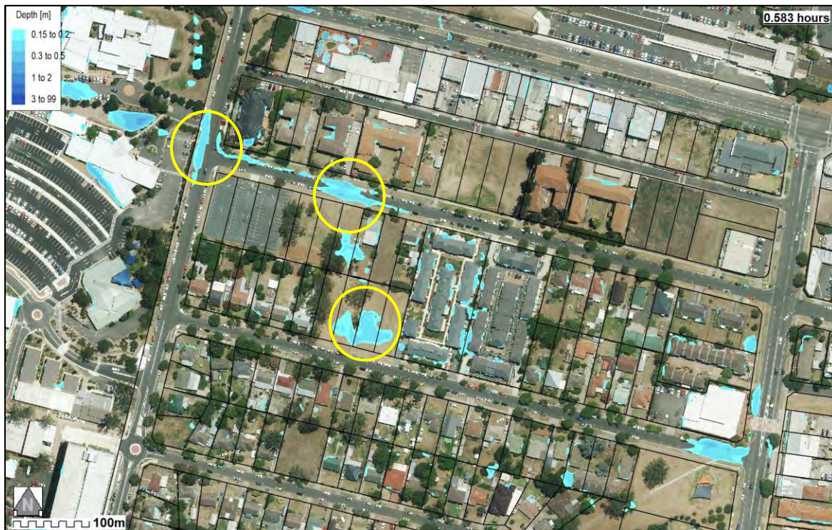
Plate 39 1% AEP Depths between Somerset and Orth Streets after 35mins of rainfall.
