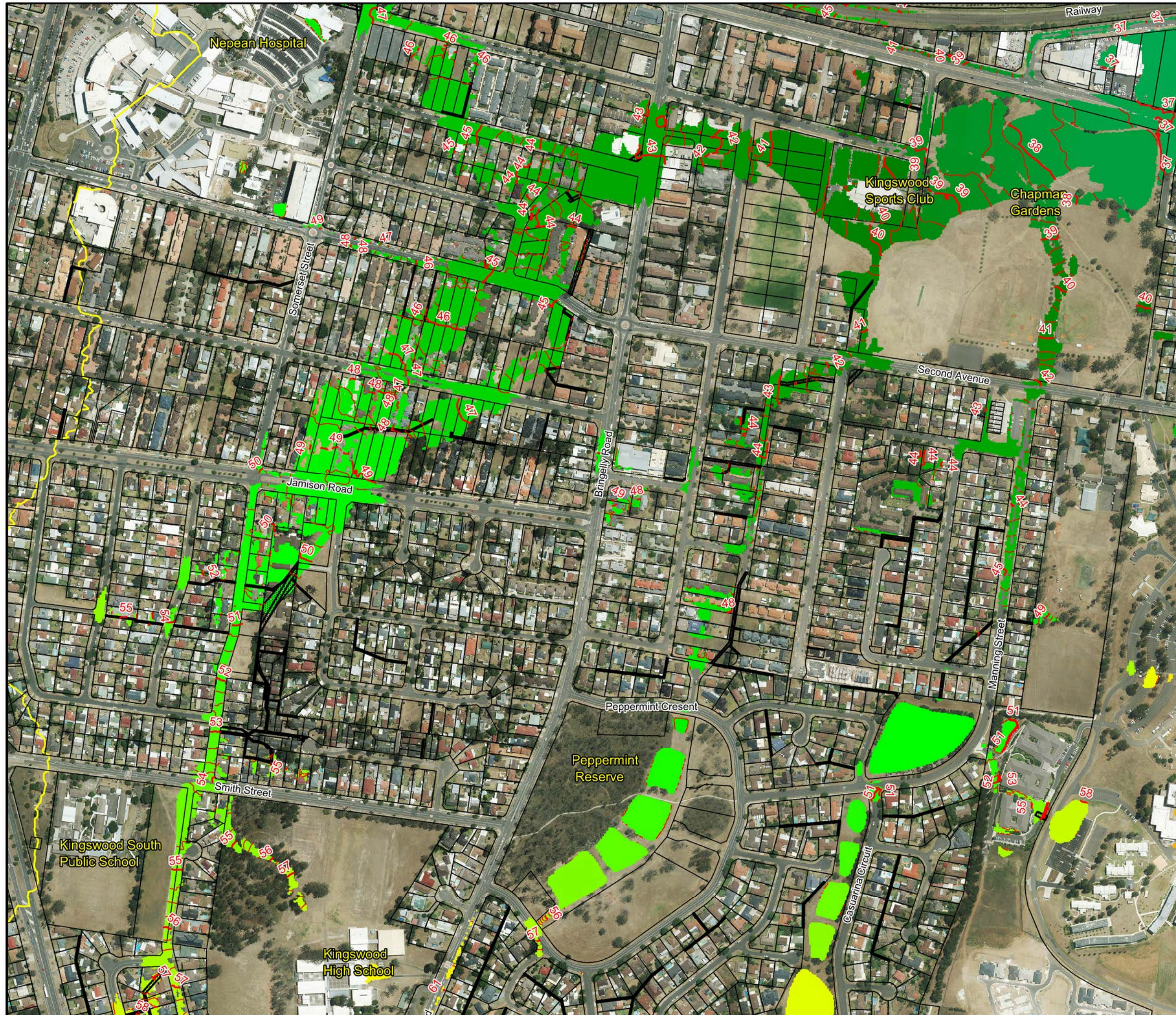
Figure 28.3: Peak Design Floodwater Levels for the 1% AEP Flood
