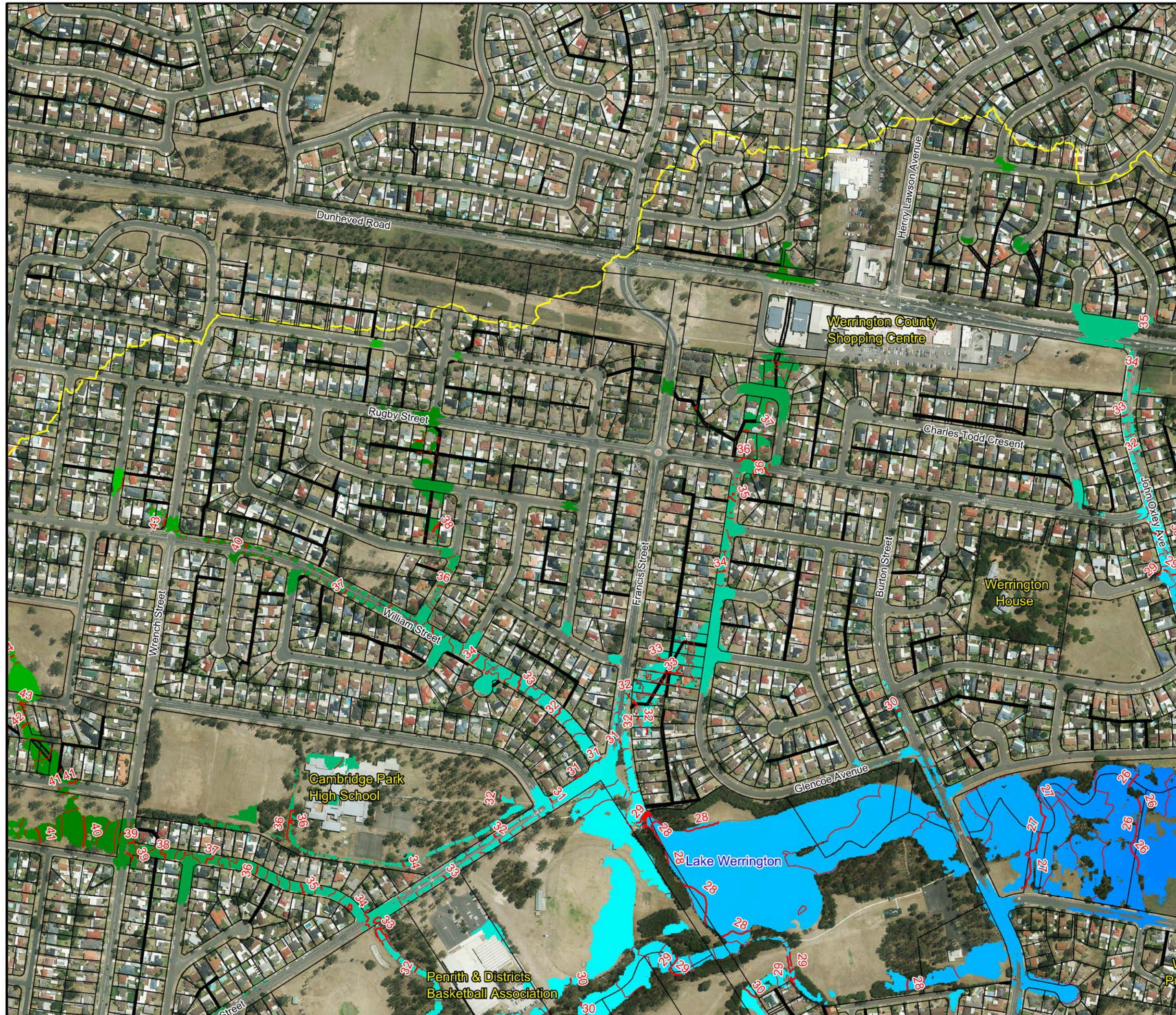
Figure 28.8: Peak Design Floodwater Levels for the 1% AEP Flood
