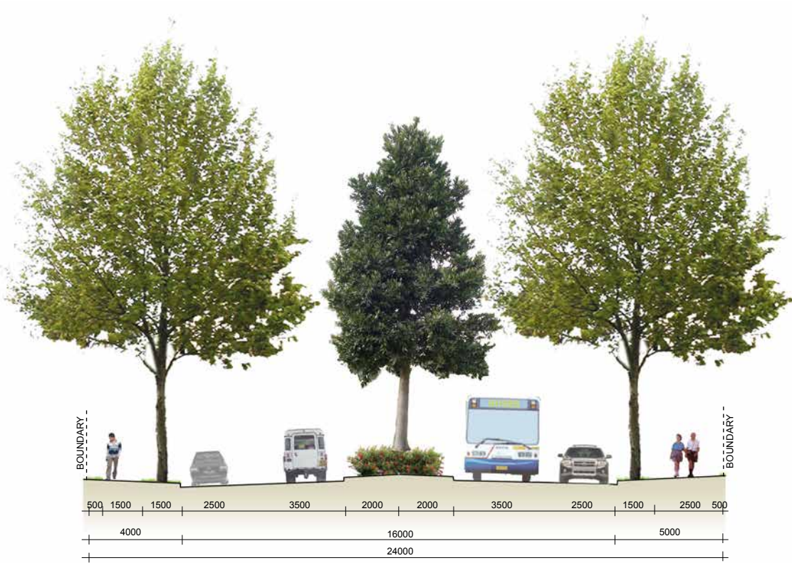
C2 - Collector Street with Median C2 Collector Street as per Precinct Plan. Off road share path adds 1m to Road reserve total width. Scale 1:200
