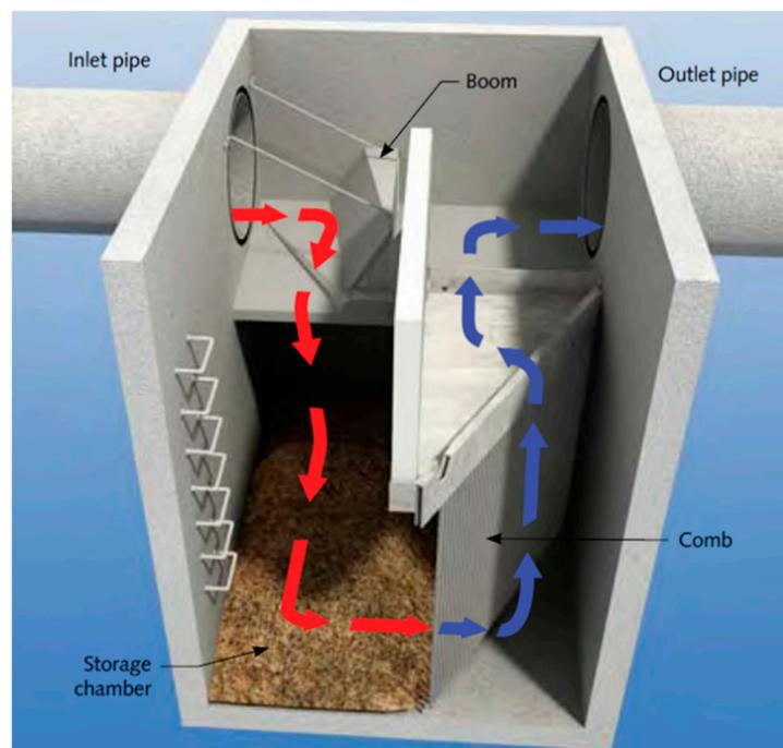
**Figure 1.** Schematic of a Humegard<sup>®</sup> GPT system showing flow of stormwater and treatment processes (Humes).
